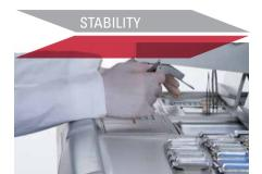
Control matters. The ergonomic wrist pads increase hand stability and precision, even when embedding the most difficult biopsies.
