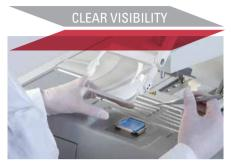
The bright white LED improves contrast and **visibility** of the most transparent samples. The user-friendly magnifier, with its wide lenses and **straightforward positioning**, helps you embed the smallest and most **complex biopsies**.
